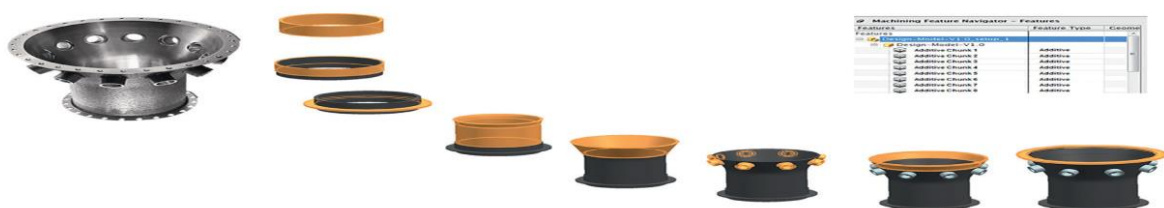
Fig. 2. Automatic and semiautomatic decomposition of parts into features for additive/subtractive operations
